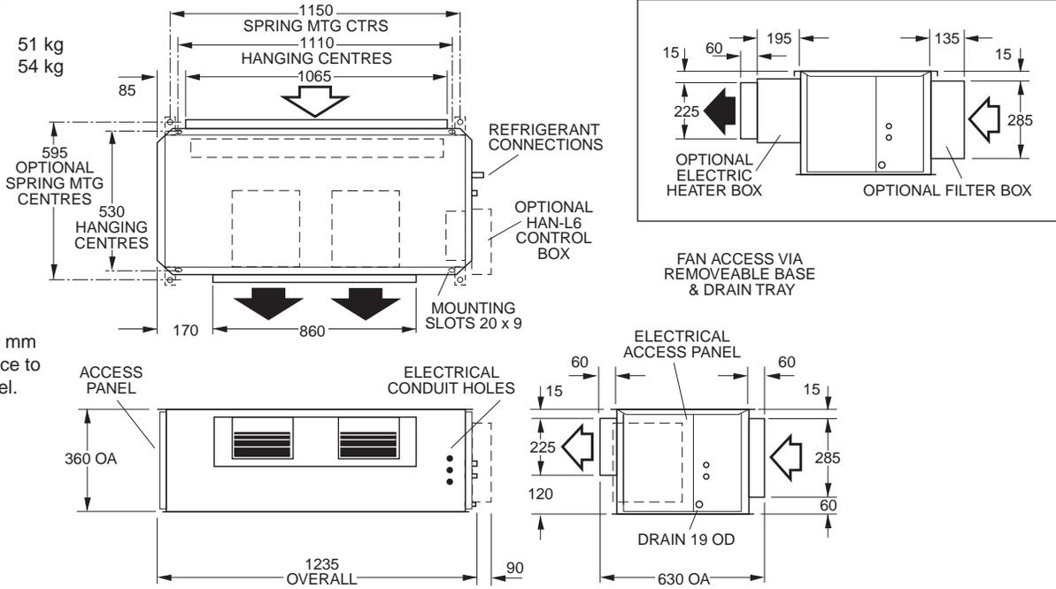
**Note :** Allow 500 mm minimum clearance to each access panel.
