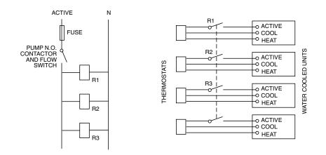
Typical Single Relay Set-Up
