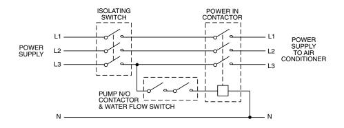
No pump running, no power supply to the units.
