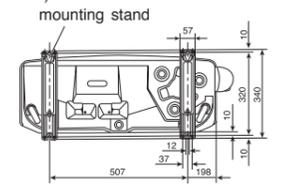
Figure showing the Installation of Outdoor Unit.
