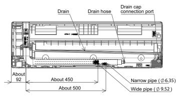
\*When piping is drawn from left side, exchange the Drain hose for the Drain cap.
