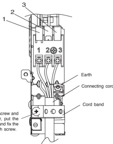
After remove the screw and the terminal cover, put the connecting cords and fix the terminal cover with screw.
