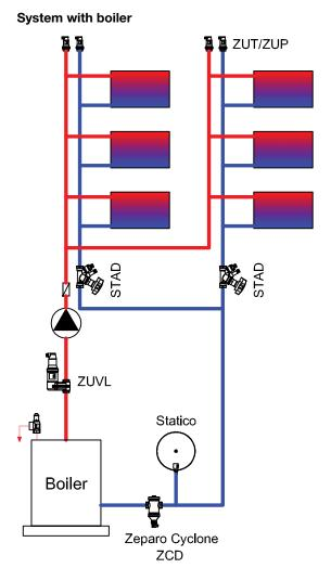
The Zeparo Cyclone dirt separator should be mounted either on the return in front of the unit to be protected or directly in front of the energy source.
