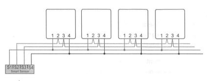
The Smart Sensor wires into the Viking's 4 smart sensor terminals located under the slide off cover at the top of the Viking controller. These terminals are labelled "Smart Sensor S1, S2, S3 & S4."
