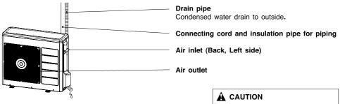
• When heating operation, drain or defrosted water flows out from outdoor unit. Don't close drain outlet portion in chilly area so as not to freeze these.
