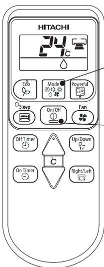
**1** Press the FUNCTION selector so that the display indicates ◊ (DEHUMIDIFY).
