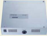
Connecting the HC-A64BNP to an H-LINK (communication line between machines) allows the use of up to 8 refrigerant cycles and control of up to 64 indoor units. Up to eight HC-A64BNP can be connected to the same H-LINK.
