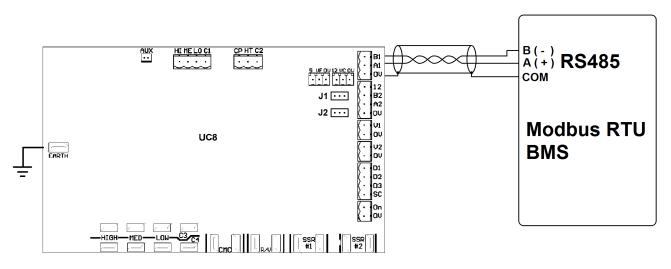
Up to a maximum of 63 units can be connected on a common RS485 bus in daisy-chain fashion.
