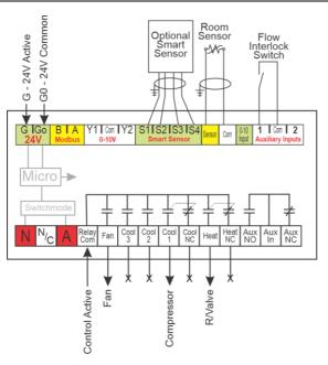
This is similar to a standard single stage heat pump except that the auxiliary input is set to shut the Viking down on loss of water, thereby protecting the system.
