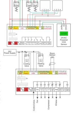
The Viking will also switch the heating and cooling relays when in Valve Mode. This permits the Viking to additionally control a circulating water pump or some other device when heating or cooling is needed.
