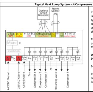
In this example the Viking is running a heat pump system with 4 compressors providing 4 stages of heating and 4 stages of cooling.
