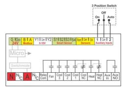
In the Auto position the Viking will run its normal 7 day or 365 day schedule. In the On position the Viking will use the "Start" program temperatures and fan mode for as long as this switch is closed. In the OFF position the Viking will shut down.
