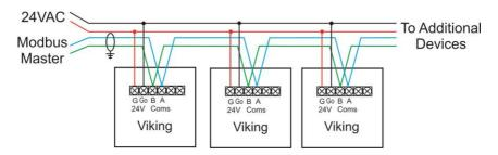
Some simple rules apply with Communications wiring; all devices MUST be in series No "T" branches or "star" wiring will be tolerated as this will seriously degrade or stop communications.
