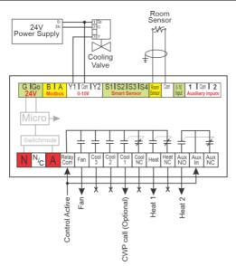
In Valve Mode both the relays and 0-10V outputs work in tandem, permitting the Viking to modulate the 0-10V valve and call for the circulating water pump on a cooling demand if required.
