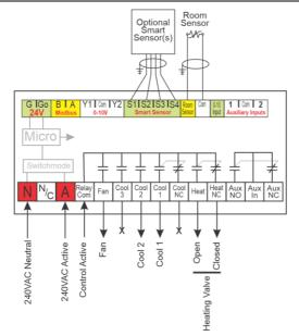
The first stage heating and cooling relays in the Viking are a changeover type permitting you to drive a heating and/or cooling valve open and/or closed.
