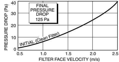
$$\text{Face Velocity} = \frac{\text{Airflow (l/s)}}{\text{Filter Face Area (m}^2\text{) x 1000}}$$
