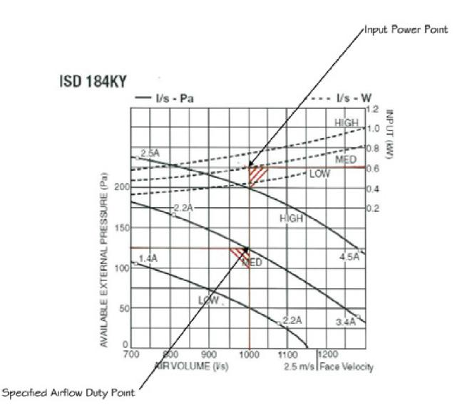
When using a Belt drive arrangement, it was not as easy to find the power input to the fan motor, until temperzone released the latest version of its USP (Unit selection Programme), which is found on our commercial web site, www.temperzone.biz
