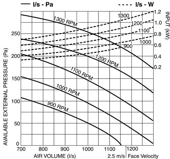
**Note:** Airflows are for a dry coil. Reduce airflow by 10% in high moisture removal conditions.
