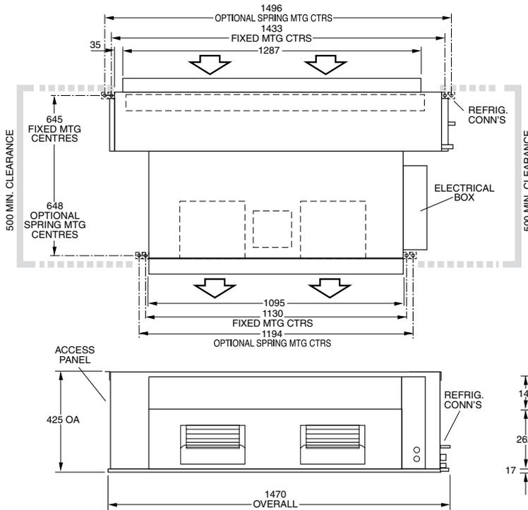
Separable for ease of installation through small man holes – minimum 550 mm sq. clear aperture
