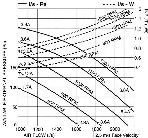
If using EU-2 filter media, provide 0.08 m<sup>2</sup> face area per 100 l/s of airflow to maximise efficiency.
