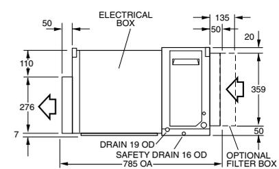
Separable for ease of installation through small man holes – minimum 550 mm sq. clear aperture
