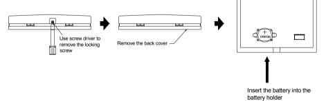
Remove and check the battery. If necessary, replace with a lithium CR2032 cell battery.
