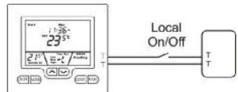
Common figure "8" (ELV Twin 0.2mm<sup>2</sup> to 0.5mm<sup>2</sup>) cable is suitable provided the sensor runs are not extraordinarily long (>30m), and that they don't run past high voltage cable or electrically noisy environments. temperzone supplies suitable wire in several lengths, 1.5m (P/N 201 000 046), 6m, (P/N 201 000 047), 12m (P/N 201 000 048), and 25m (P/N 201 000 049).
