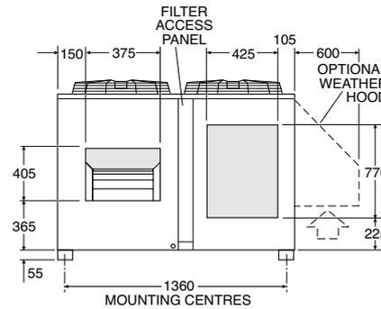
**Fig. 2 Downward Supply Air / Mounting Rails Version 2**
